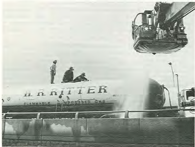
Above: Illustration of plug that was used to seal the offending leak. Below: Heroic members of Rescue Co. 4 at work, actually sealing the leak. Fog curtains, supplied by handlines, Stang nozzles, and a tower ladder protected the area throughout the operation. It was this concerted and dedicated F.D. effort that averted disaster and brought this operation to a successful conclusion.
