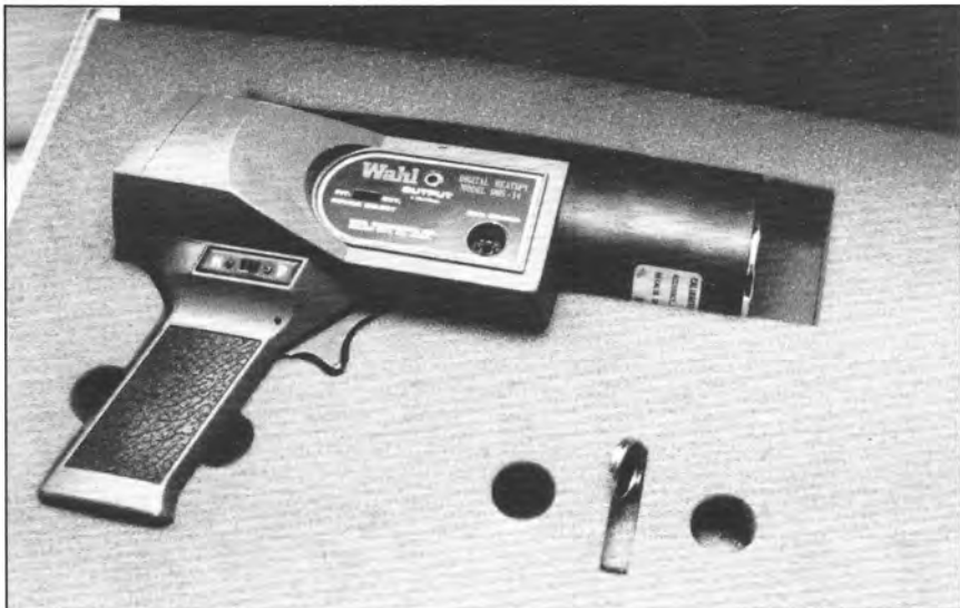
The Wahl Heatspy infrared thermometer gives a digital readout in Fahrenheit and centigrade.
