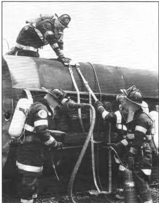
. . . as part of a patching, metering, grounding, off-loading and foam back-up operation.
