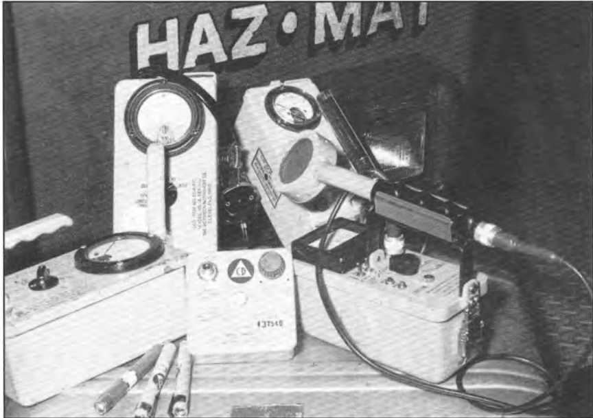
Radiological equipment includes: left, a Victoreen Geiger counter, model CDC-700; rear, two Victoreen survey meters, model CDV-715; right, a Ludlum detection meter, model 14C, with a pancake probe; center, a dosimeter charger and assorted dosimeters.
