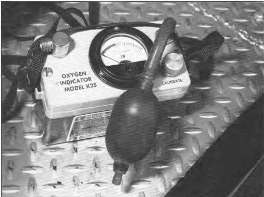
A manual, pump-operated oxygen indicator measuring in percent determines oxygen displacement or enrichment.
