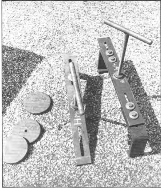
Dome-cover clamps used to secure the hatch covers on overturned gasoline or oil trucks.
