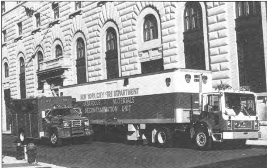
FDNY Mobile Decontamination Truck, right, housed at Ladder Company 15 in Manhattan. The unit contains four hot-water showers, a facility to catch the run-off water, and dressing rooms for final decontamination. The support vehicle carries tarps, coveralls, plastic bags, hoses, recovery drums and other items necessary to putting the Decontamination Truck into operation.
