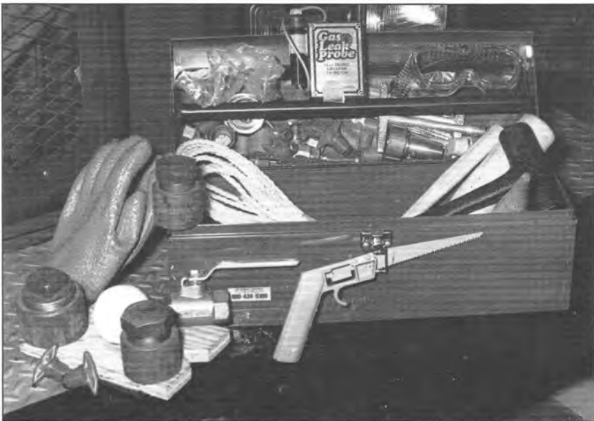
A propane leak-seal field test kit includes an electronic gas leak detector (top center) and assorted fittings and tools.
