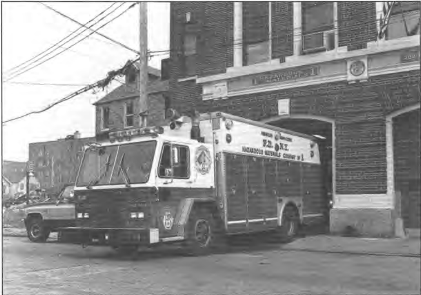
Haz-Mat's first vehicle, a 1983 American LaFrance with a Saulsbury box, was retrofitted to fit their needs.
