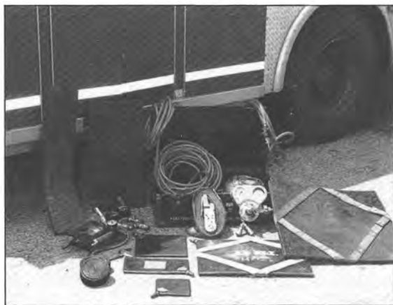
Maxi-force air bags, providing low lift but able to endure high pressure.
