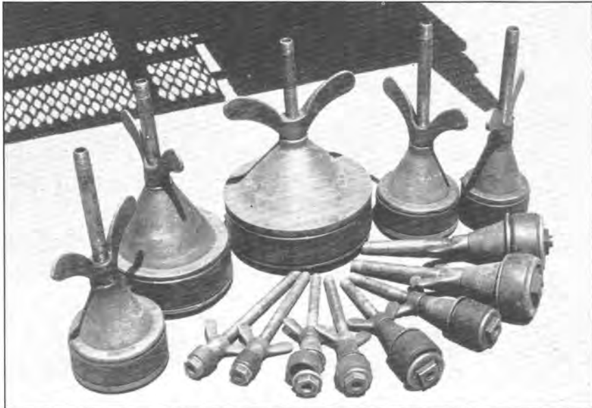
Various sizes of boiler plugs add to Haz-Mat's leak-stopping capability.
