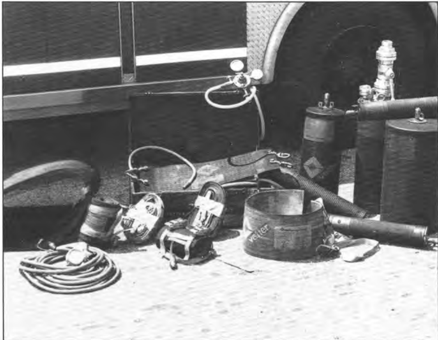
Vetter low-pressure leak seal kit with various sizes and shapes of patches and plug bags which can be pressurized either pneumatically or with water.
