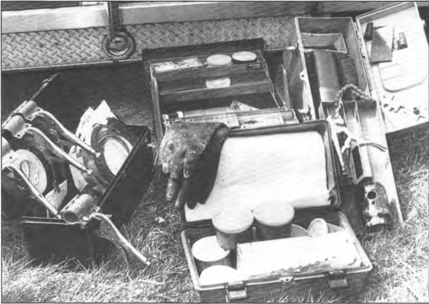
Leak-seal kits include plugs, clamps, epoxy, magnetic-patch kits, gaskets, duct tape, and much more.
