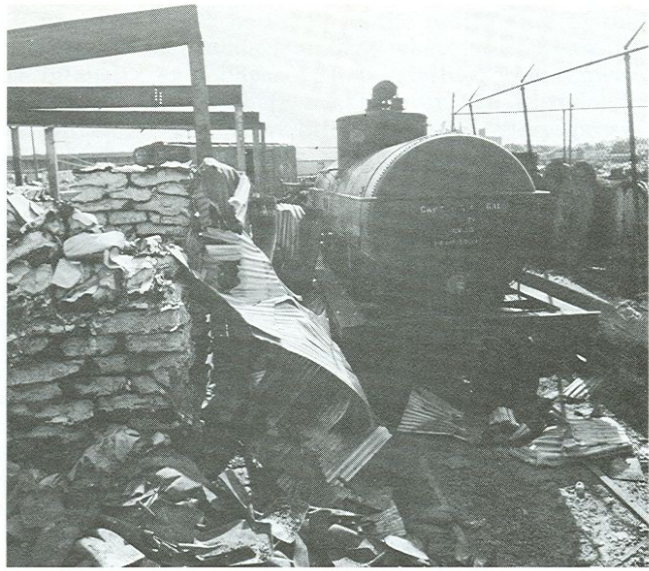
Tank car, containing 4,000 gallons of diesel oil, remains unharmed. Members of L.135 employed their heavy calibre stream to create a protective water curtain for the tank car, keeping it safe.
