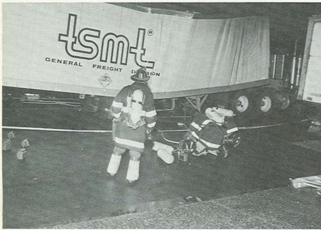
Above: Capt. Joseph Gallagher, Haz Mat unit, supervises placement and inflation of Lo-Pressure Vetter Lifting Bags under damaged truck.
