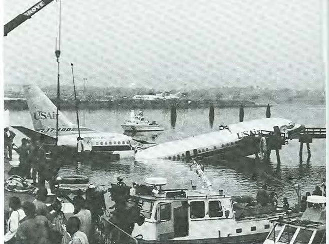
When salvage began, the tail was lifted using an arrangement similar to the one Rescue 5 had used to stabilize it during the search for the black box. Photo courtesy of The New York Post
