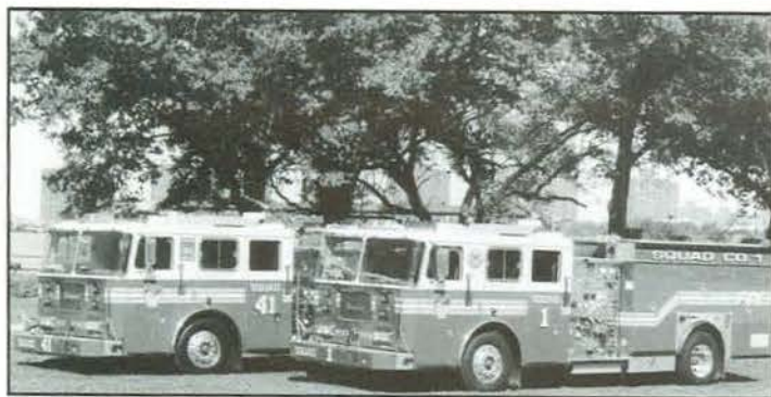
Squad Companies 1 and 41 operate 1000-gpm rescue-pumpers, equipped with additional compartments to carry assigned equipment.
