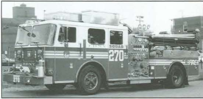
The remaining Squads operate conventional pumpers that have been modified with additional compartments and large equipment boxes.
