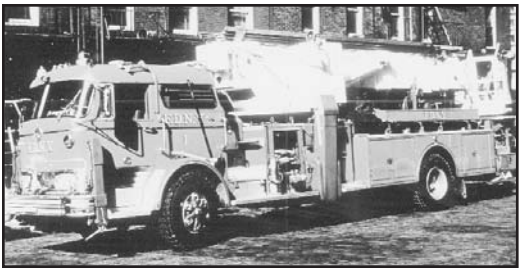
Mack Trucks developed the first tower-ladder in 1964, in conjunction with FDNY, to meet specific design and operational criteria common to New York City. The tower-ladder revolutionized firefighting procedures in New York.
