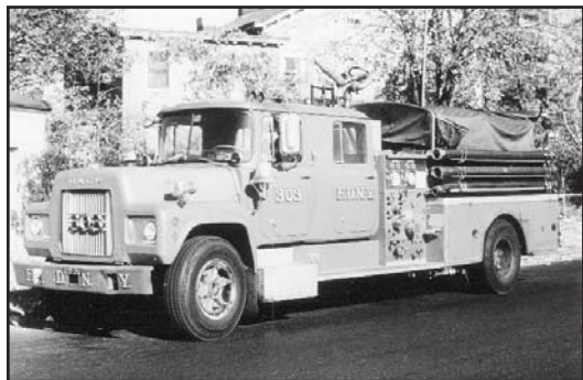
Following widespread civil unrest, the Department sought to provide a higher degree of protection to firefighters than was offered by open-cab apparatus. The first attempt at a crew cab design was a modified highway maintenance truck design. These apparatus proved less than desirable and the cab-forward model was redesigned into a crew cab.
