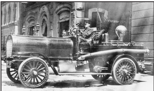
FDNY's first motorized pumper was this 1911 Waterous 750-gpm unit assigned to Engine 39. While the motor took up a good portion of the apparatus, the pump took up the remainder and is positioned behind the seat. There was no space on the pumper to carry hose and separate hose wagons were required.
