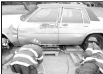
Air bags have proved their usefulness many times, lifting odd-shaped objects, to effect rescues.
