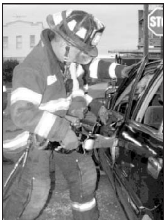
Firefighter employs Hurst Tool to spread car doors to rescue a trapped victim.
