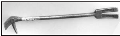
The Halligan Tool has myriad uses and provides firefighters with a lightweight, strong tool with a solid feel.
