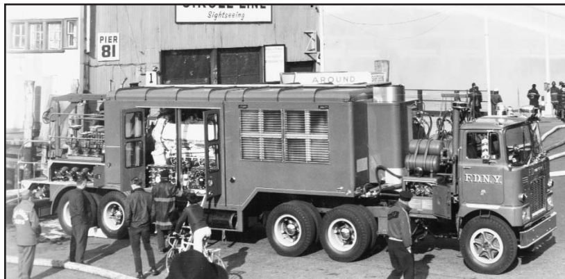
The Super Pumper system was purchased to address water problems encountered at brush fires.
