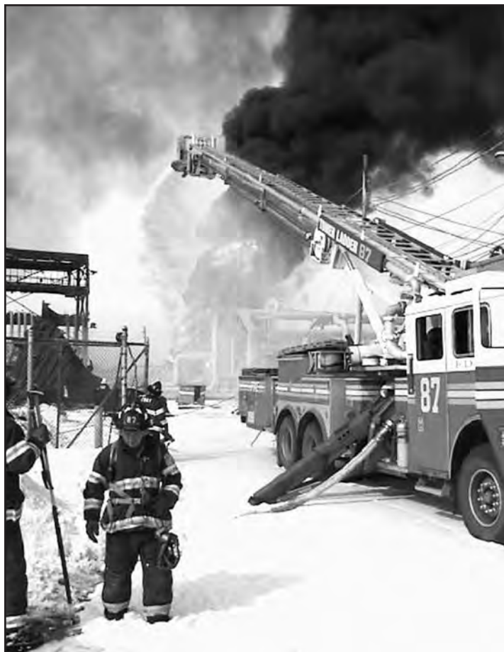
Tower Ladder 87 directs its Angus foam cannon at the burning product manifold.
