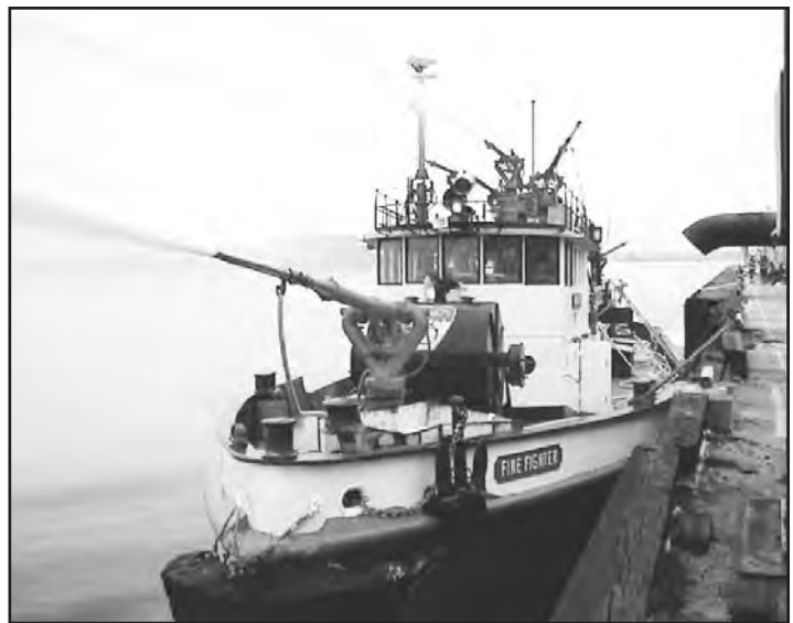
Marine Co. 9 uses water monitors to break up floating fuel and cool remains of the sunken barge, while a 1000-gpm Angus foam cannon on the bow monitor is supplied with foam concentrate from a portable 600-gallon reservoir on its foredeck.
