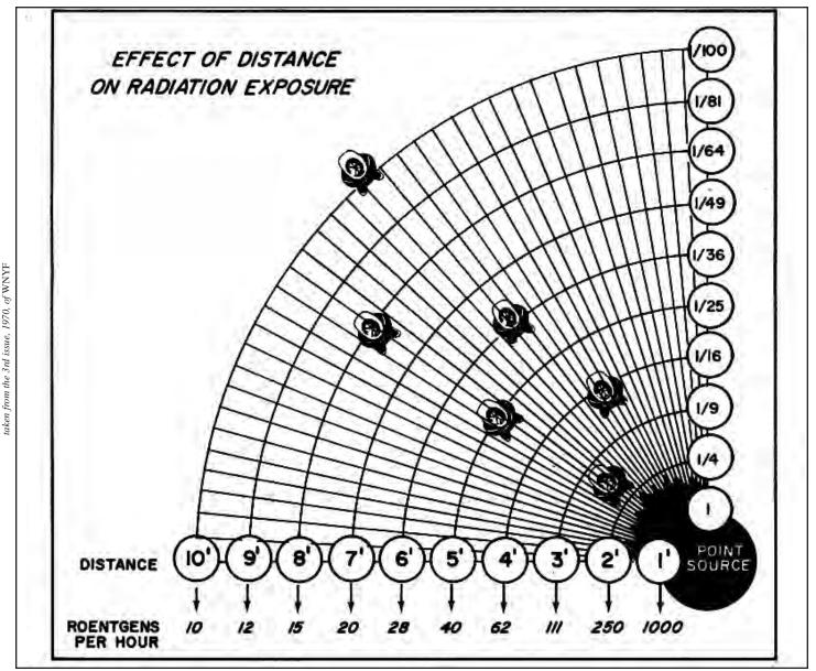
This chart shows the concept of the lessening of radiation intensity at various distances from a point source. It can be seen that there is a dramatic "fall off" in the rate of exposure as a person moves away from the source of radiation. Even a little distance from the source is very significant in increasing the safety factor. Conversely, as the distance is closed to the radiation source, the levels of radiation exposure go higher by the same mathematical process.
