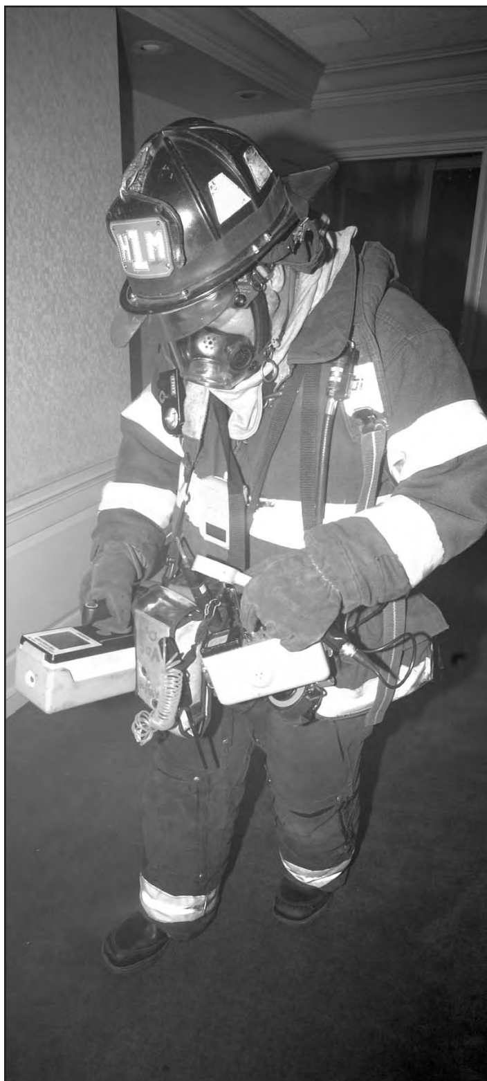
Haz-Mat 1 Firefighter employs a Rad-50 radiation detector during FDNY high-rise drill that featured incendiary devices and radiological material as weapons to create a dirty fire.
