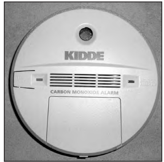
Figure #1--A battery-operated carbon monoxide alarm with no digital display.
