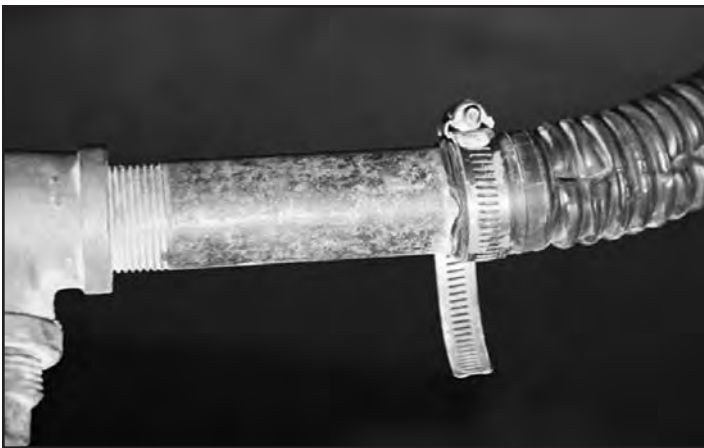
(Above) Hose connected to nipple. This is the bottom part of the illegal connection shown on page 5. (Below) Hookup in street.
