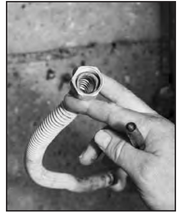
(Left) Close-up of uncompromised threads of stove #1. (Right) Uncompromised threads on connection of stove #2. Both were disconnected (as opposed to blown apart by an explosion), showing evidence of tampering.
