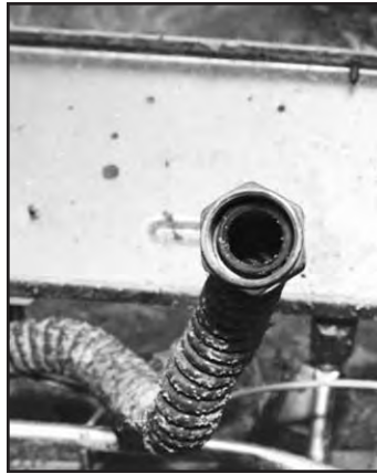
(Left) Close-up of uncompromised threads of stove #1. (Right) Uncompromised threads on connection of stove #2. Both were disconnected (as opposed to blown apart by an explosion), showing evidence of tampering.
