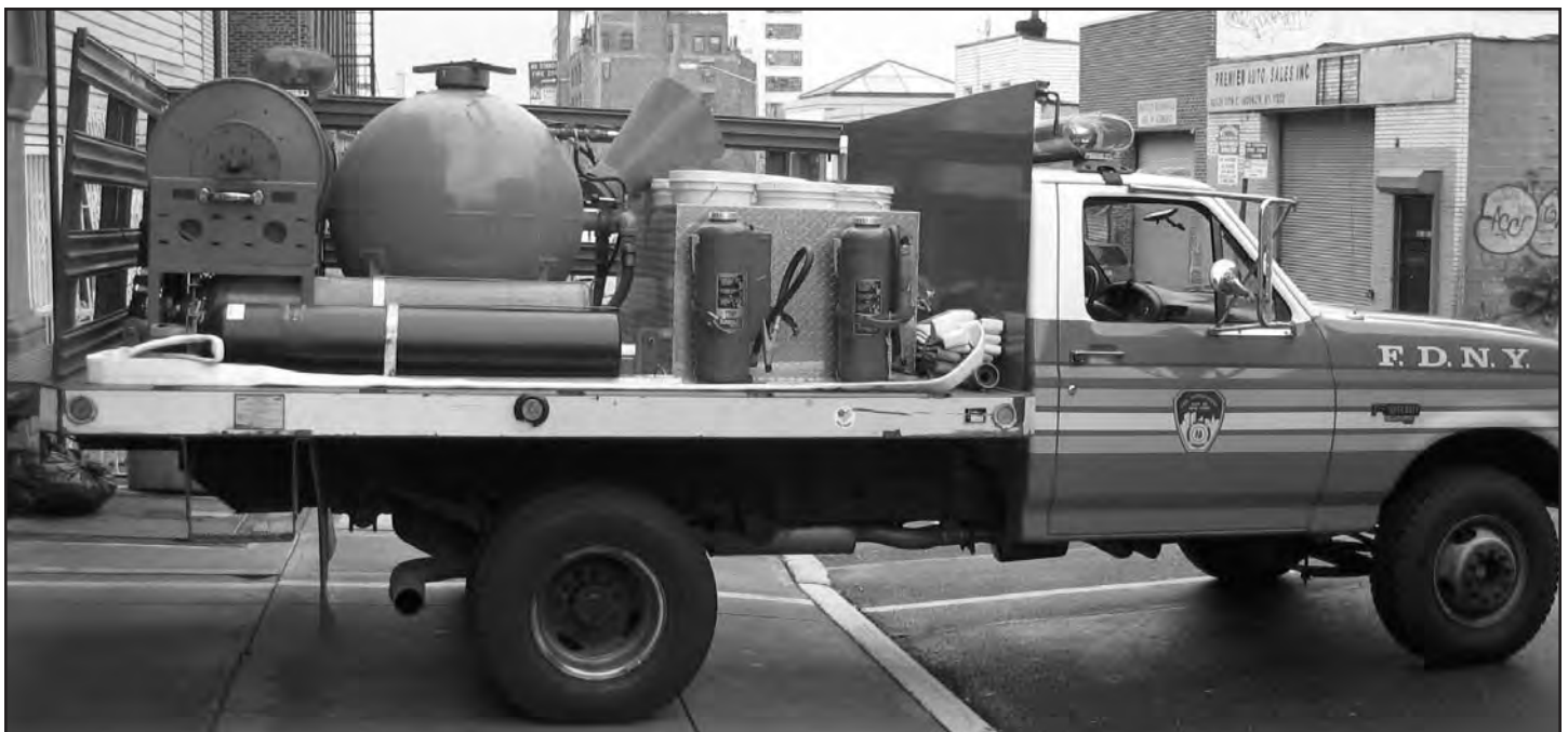
The Purple K unit of Engine 228, one of the original units introduced in 1997. It carries 700 to 750 lbs. of Purple K.
