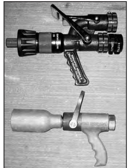
The two nozzles carried on the Purple K units. The top nozzle is a dual hydro-chem nozzle, which gives the unit the capability of providing foam and dry chemical powder through the same nozzle, either simultaneously or independently. The bottom nozzle is a 1 1/4-inch straight-bore nozzle, which distributes the powder in a wide pattern.
