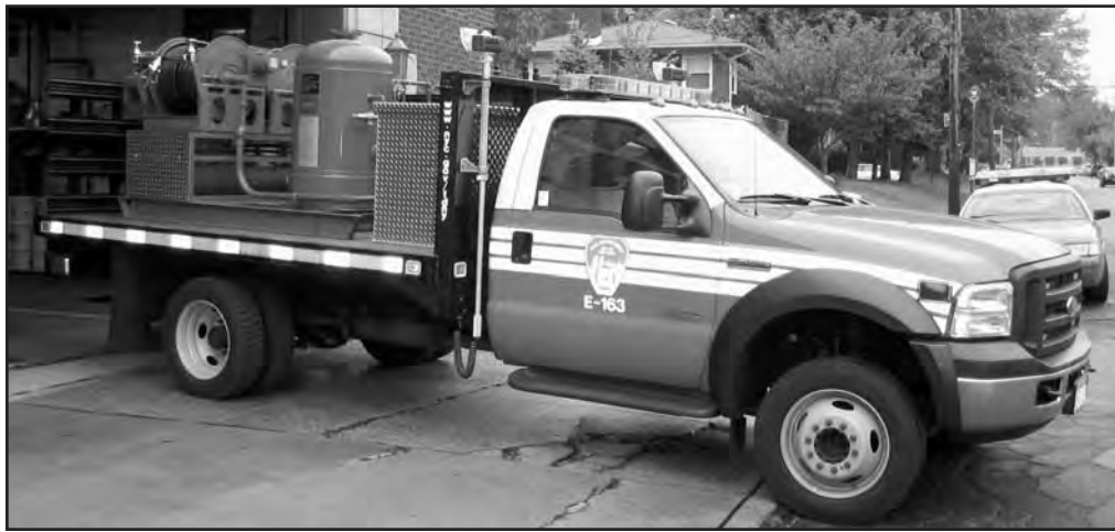
The Purple K unit of Engine 163. This newer unit contains 1000 lbs. of Purple K powder and increases members' operational time slightly.
