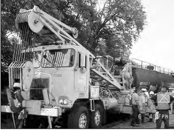
Heavy equipment was brought in to lift the propane car back onto the tracks.
