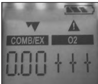
Excess O 2 is indicated by the “+++.” An explosion or fire hazard exists.
