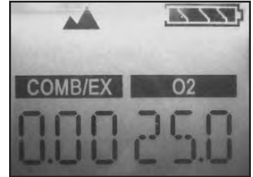
Peak readings page on MSA Altair Meter permit viewing of high readings.
