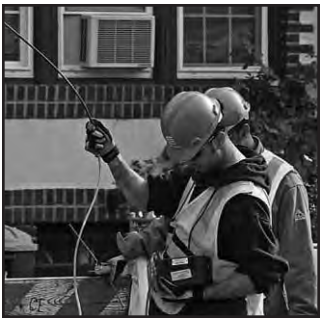
(Left) ConEd employees use a GMI Gasurveyor 3 (a close-up of which is pictured at the right).
