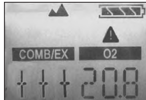
Excess combustibility is displayed in the percentage LEL of combustible gases.
