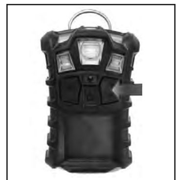
Reset button (arrow) on MSA Altair Meter acknowledges and silences alarms.
