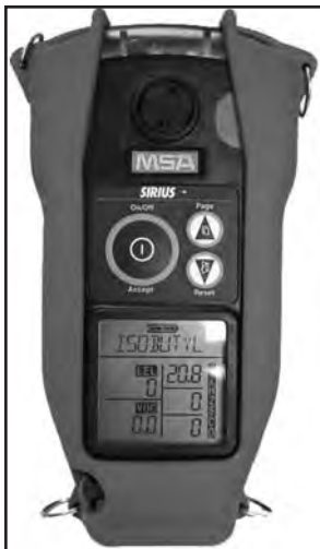
MSA Sirius (left) and Five Star (right) Meters are combustible gas indicators that are carried by SOC units. The meters are calibrated with pentane to provide accurate LEL readings.
