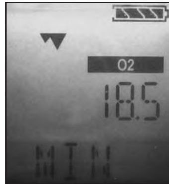
Minimum oxygen page on MSA Altair Meter reveals the lowest oxygen reading.
