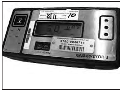
(Left) ConEd employees use a GMI Gasurveyor 3 (a close-up of which is pictured at the right).
