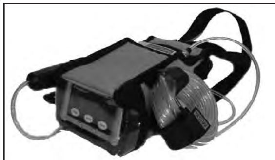
MSA Sirius (left) and Five Star (right) Meters are combustible gas indicators that are carried by SOC units. The meters are calibrated with pentane to provide accurate LEL readings.
