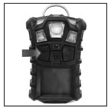
Page button (arrow) on MSA Altair Meter shifts through data screens.
