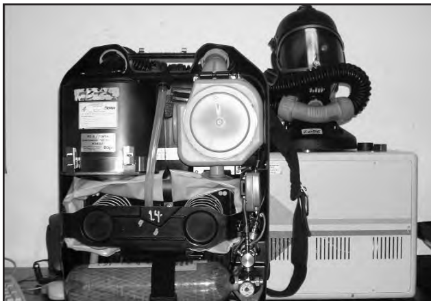
(Left) Rear view of Draeger BG-4 Extended Duration SCBA (EDSCBA). (Above) Internal components of the EDSCBA. (Right) Note the slim profile of the Rebreather.
