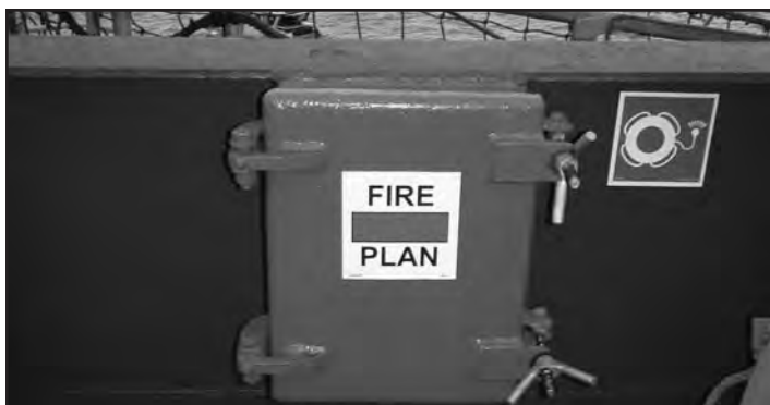
The ship's fire safety plan usually is found in a weather-tight box, adjacent to the gangway on either side of the ship.
