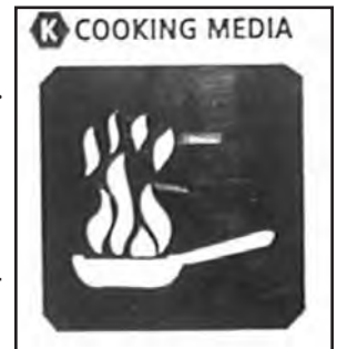
(Left) Portable (Class K) wet chemical fire extinguisher with unique wand applicator. (Above) Wall-mounted releasing mechanism and pressurized wet chemical cylinders. (Right) Class K (wet chemical agent) portable fire extinguisher pictogram.
