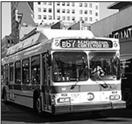
Photos #1 and #1A, left and above--Long cylinders on top of the bus identify it as a CNG (compressed natural gas) bus.
