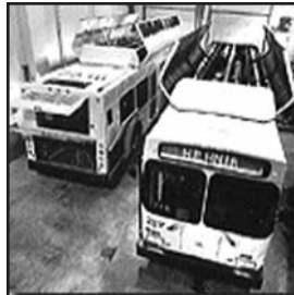
Photos #1 and #1A, left and above--Long cylinders on top of the bus identify it as a CNG (compressed natural gas) bus.
