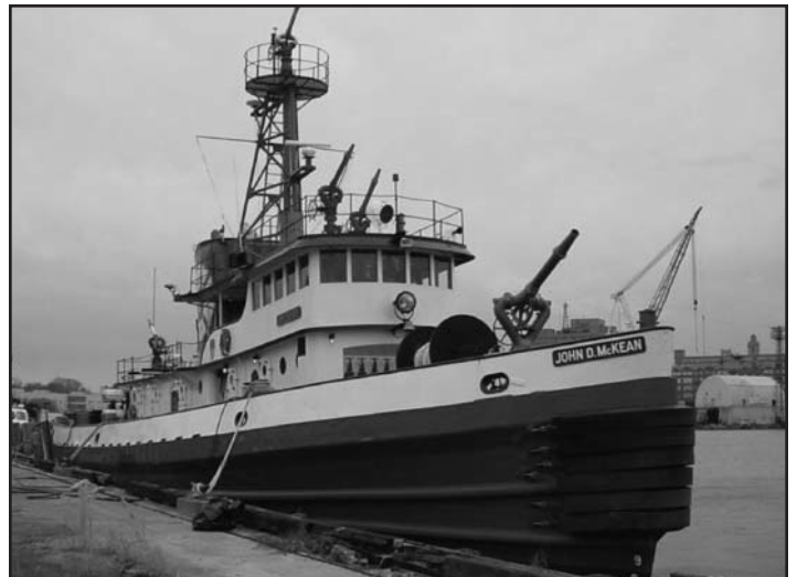
The John D. McKean was replaced with the Three Forty Three —a high-performance, 140-foot fireboat that features the Harbor's inter-agency command and control platform.
