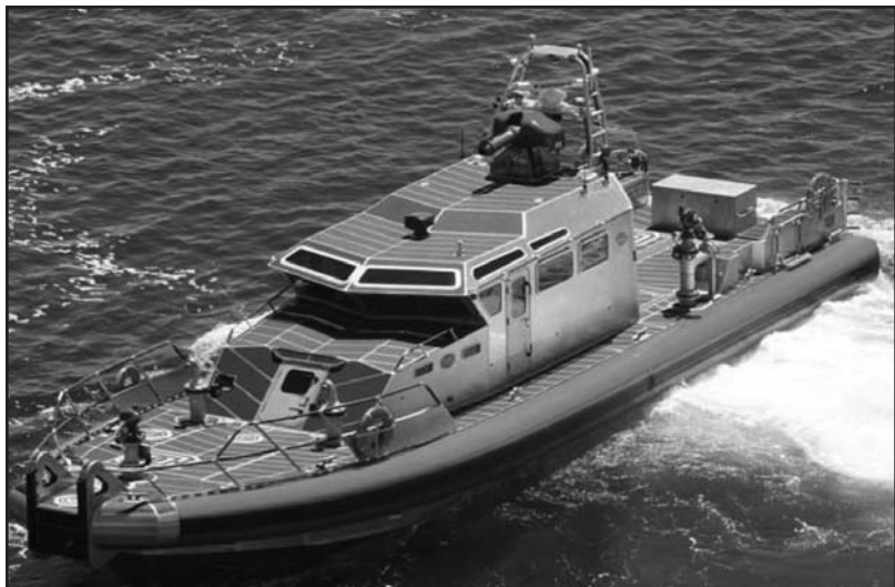
The high-performance, 65-foot fireboat, The Bravest , features 50-mph, triple 1000-hp jets and pumps 6000 gpm.
