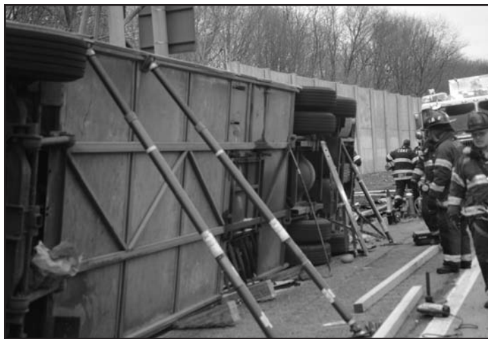
Photo #4--Members of Rescue 4 and Ladder 27 provided the shoring to keep the bus safely on its side. This operation was coordinated by Battalion Chief Donald Hayde, Rescue Battalion.
