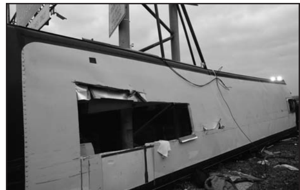
Photo #3--Enlarging the bus' roof hatch to four by seven feet facilitated removal of victims by Firefighters.
