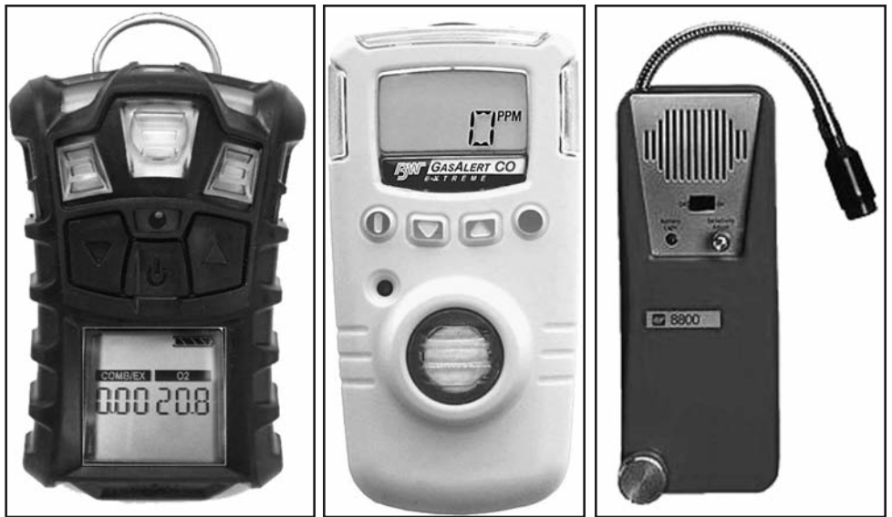
Left to right are the meters carried by FDNY Firefighters: MSA Altair Meter, BW Technologies GasAlert Extreme CO Meter and the TIF 8800 Combustible Gas Detector. For detailed information regarding these individual meters, members are urged to review "Introducing the MSA Altair Multigas Meter," by Captain Carlos Vazquez, in the 1st/2009 issue of WNYF.
