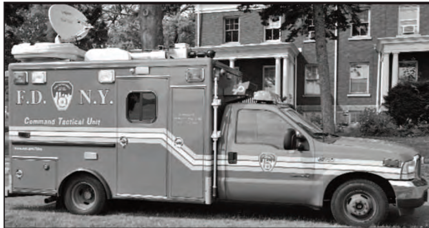
Using cameras, a network system and satellite dish, the CTU is a refitted ambulance that provides vital information to the Incident Commander.
