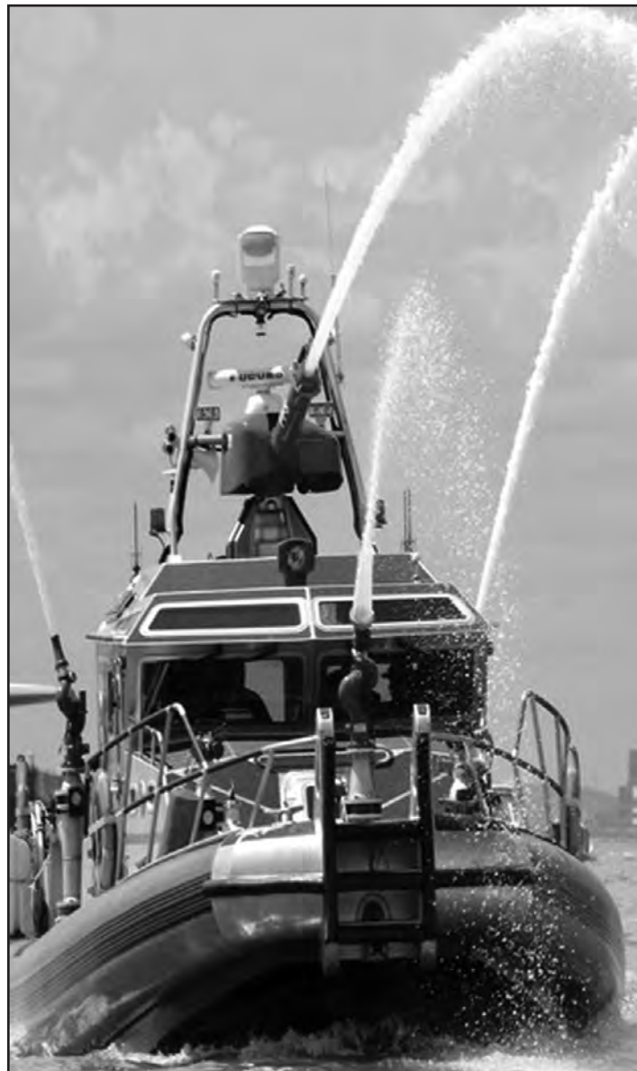
The Bravest is a high-performance, 65-foot fireboat. It features 50-mph, triple 1000-hp jets and pumps 6000 gpm.
