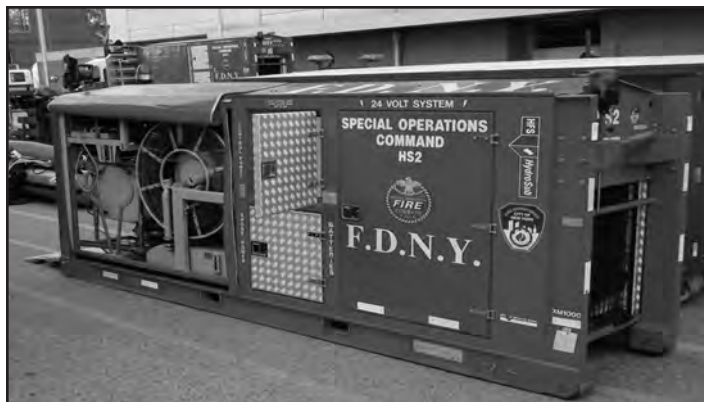
The Hytrans pumps serve as an alternate water supply source when hydrants are unavailable or malfunctioning.
