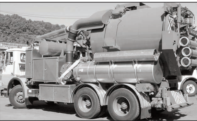
Con Ed vacuum truck shown with suction boom and eight-inch aluminum extensions. Two of these trucks were used on March 19, 2013, at Manhattan Box 1233 to facilitate removal of the victim trapped in the Bull's liver.
