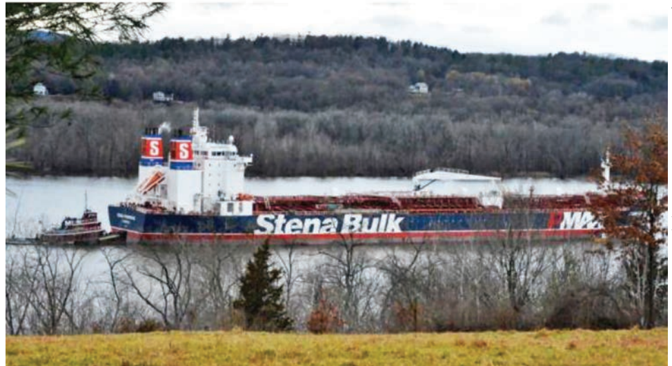
The Stena Primorsk ran aground in the Hudson River on December 20, 2012. However, none of the 12 million gallons of oil it was carrying was lost, thanks to the oil tanker's double-hulled design.
