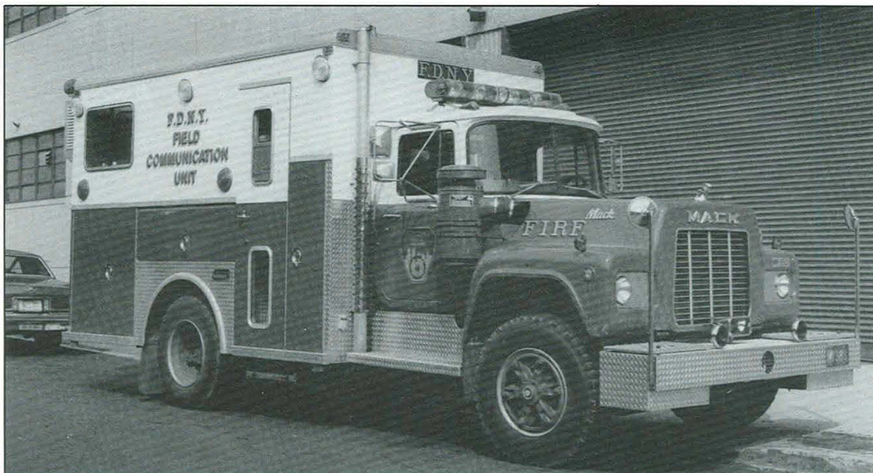
Field Communications Unit 1 operates this short wheel base Mack with custom built Saulsbury body that is equipped with an array of communications equipment. photo by John A. Calderone
