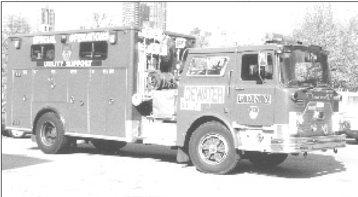
The Utility Support Unit, commonly known as the De-watering Unit, is equipped with numerous pumps, smoke ejectors and related support equipment and is capable of sustaining a large-scale de-watering operation. photo by John A. Calderone
