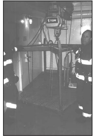
Hoist was used to remove victim from the vehicle deck to the ship's "top" deck.
