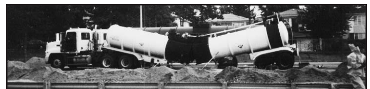
The Haz-Mat 1 team used a Vetter low pressure-high lift air bag to support the rear tank.
