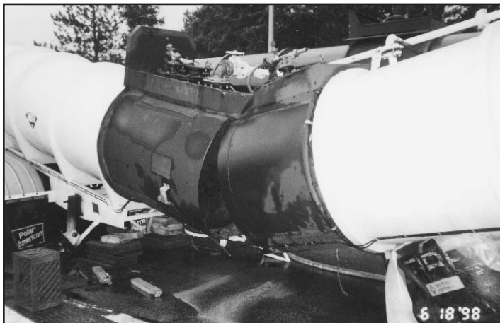
Rescue 5 members employed cribbing to support the front tank area. photos this page by Tom Ingram
