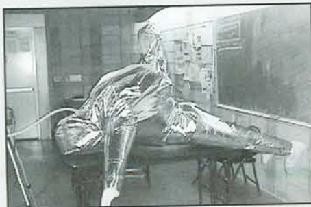
Inflation (pressure) testing of level-"A" suit.
