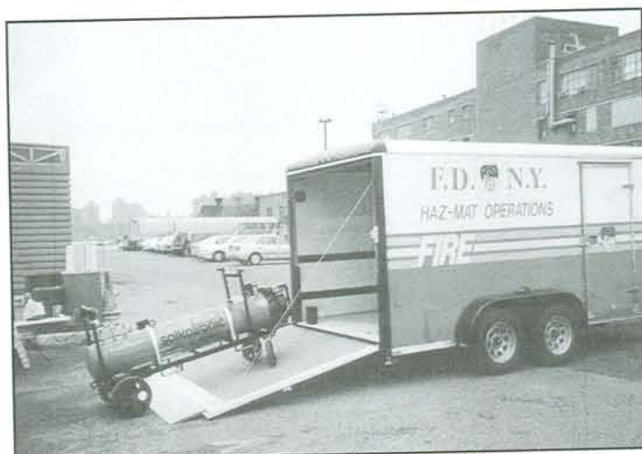
Containment vessel trailer.
