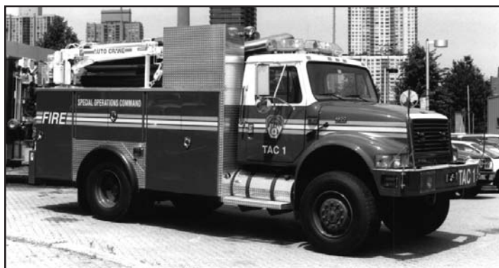
The Tactical Support Units have four-wheel-drive capability and are equipped with a front-mounted winch, generator, crane and light tower.
