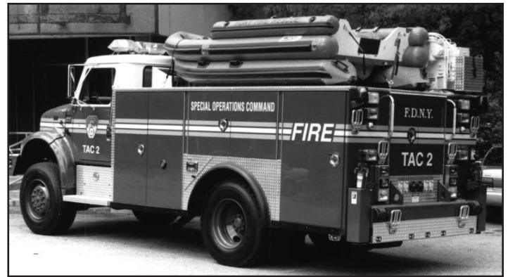
Rear view of the Tactical Support Unit shows the outriggers, electrical supply outlets and rescue boat.
