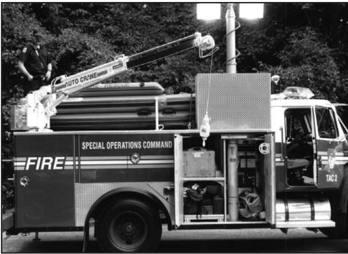
The crane has a 10,000-foot/lbs. capacity: three-foot reach @ 3200 lbs. to 15-foot reach @ 660 lbs.
