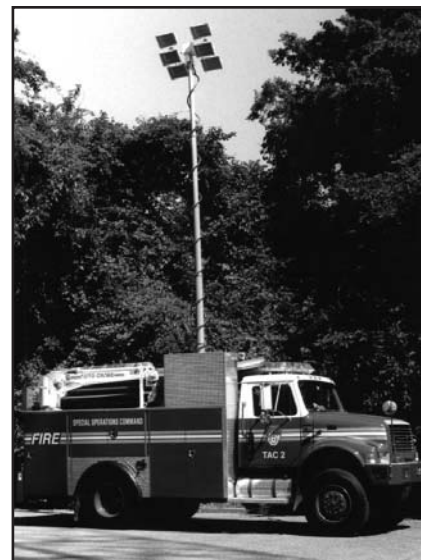
The light tower extends to a height of 30 feet and is capable of turning the operations scene into a safely lit area.
