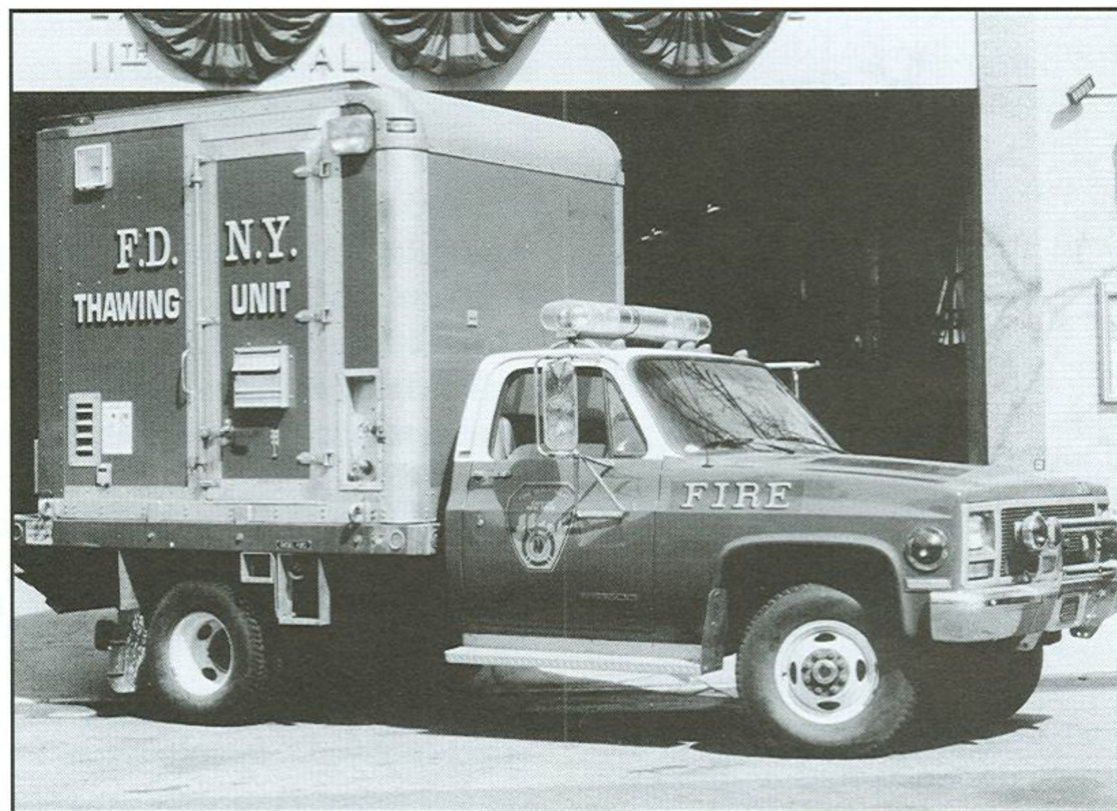
Thawing Units 1 and 4 are assigned 1989 GMC four-wheel-drive apparatus. These have skid-mounted bodies that easily can be removed and remounted on other flatbed chassis.
