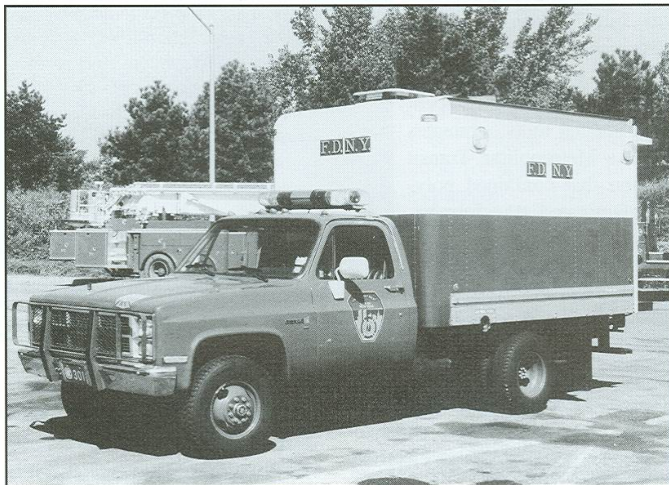
Older-type thawing apparatus are assigned to Thawing Units 2, 3 and 5. They are 1984 GMC four-wheel-drive units that were outfitted by the Shops.
