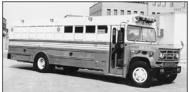
The Shops converted this GMC school bus chassis, formerly a personnel carrier, for MERV 4.
