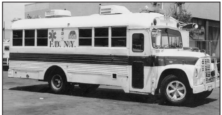
MERV 2 employs a modified International school bus chassis.
