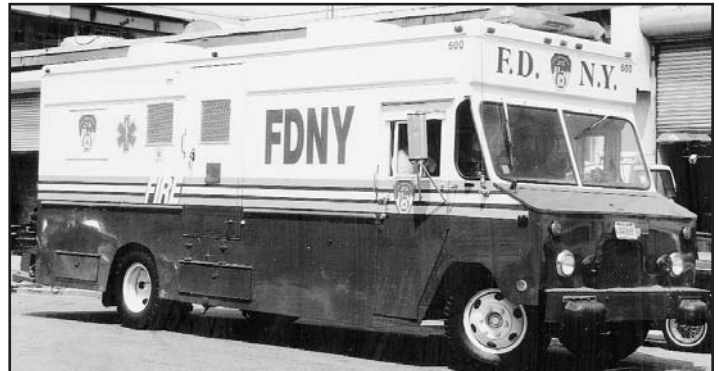
A stretched delivery van chassis was modified as the apparatus of MERV 3.
