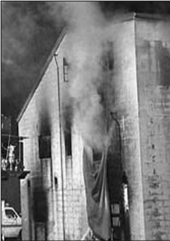
(Above--Curtain Down to Vent) After the fire is knocked down and the area is thoroughly cooled to prevent reflash as fresh air is admitted, the curtain may be raised or lowered to facilitate venting the area.
