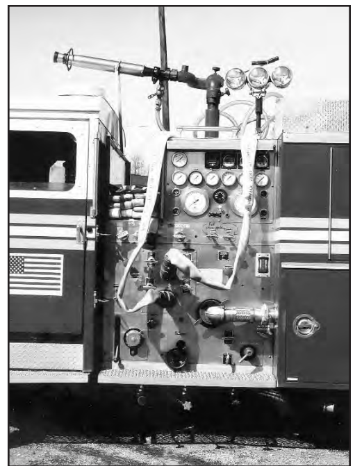
(Right) The converted apparatus features a 1000-gallon poly-tank and a foam deck pipe.
