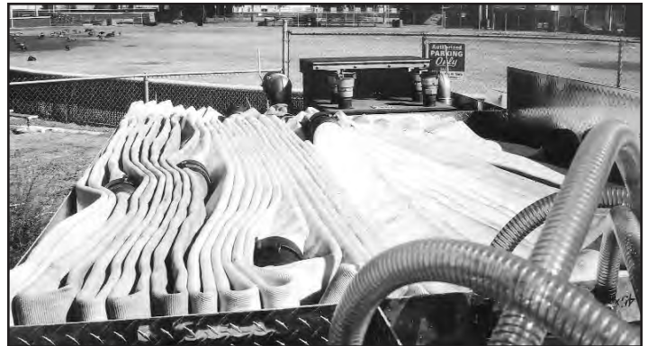
(Above) Some of the 3 1/2-inch hose used for a water supply-line in the reconfigured hose bed.
