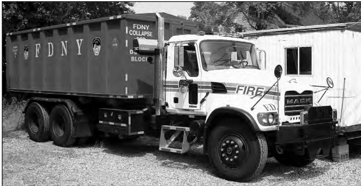
Two roll-off trucks have entered service to transport 10 collapse pods that are pre-positioned throughout the City.
