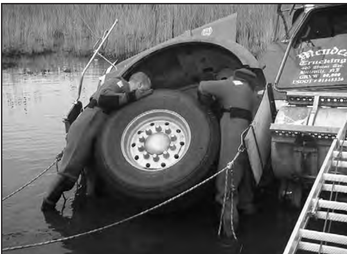
Wearing exposure suits, FDNY members prep the vehicle in the process of uprighting it. Ultimately, three heavy-duty wreckers removed the truck from the water.
