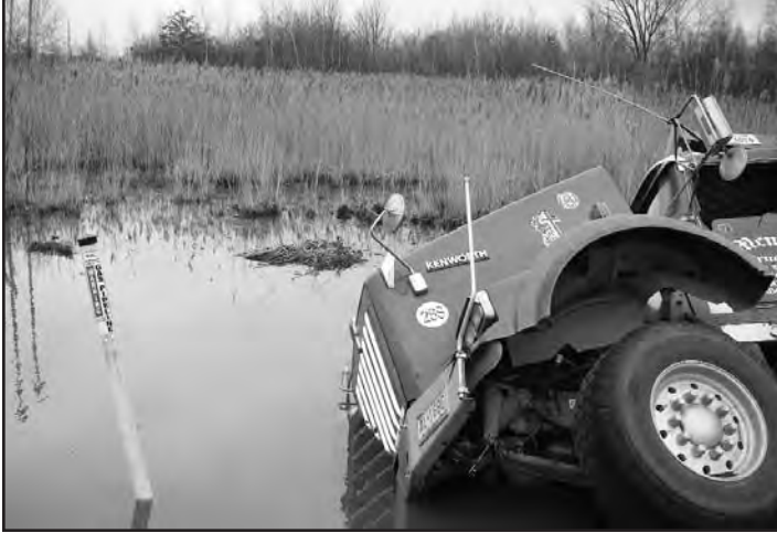
Markers indicated the presence of multiple pipelines.
