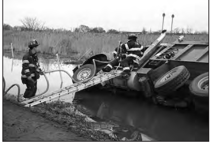
Diesel fuel is off-loaded by FDNY members. Two pipelines were bowed under the truck's weight.
