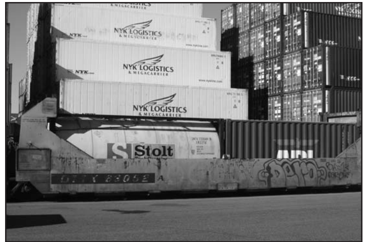
Photo #4--Rail car carrying an IM tank and an ISO container.
