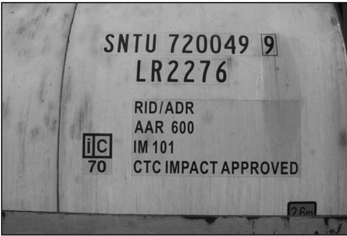
Photo #3--Intermodal tank displays typical reporting marks and numbers.
