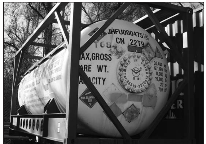
Photo #2--An intermodal Spec-51, containing refrigerant gas 134A.
