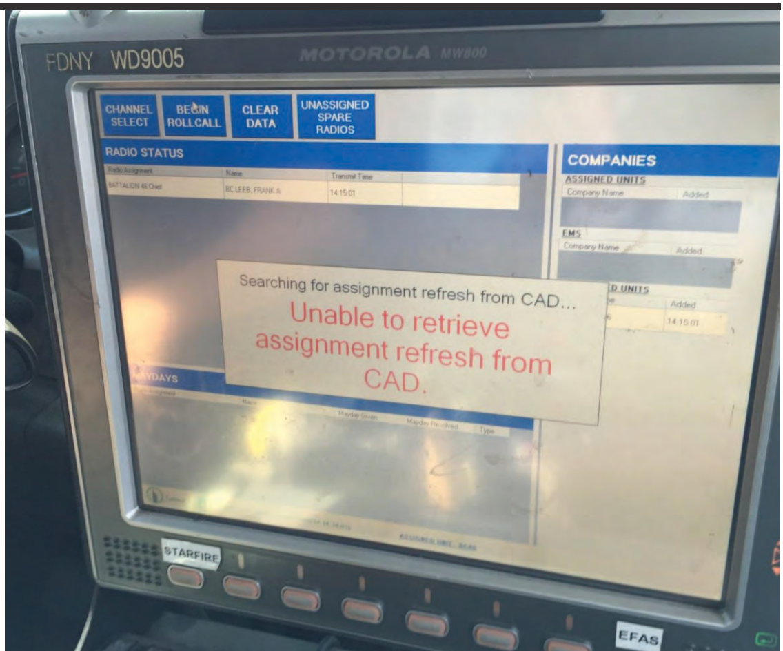
Photo 7—EFAS screen in the "begin roll call" screen when the system is unable to retrieve assignment from CAD.
