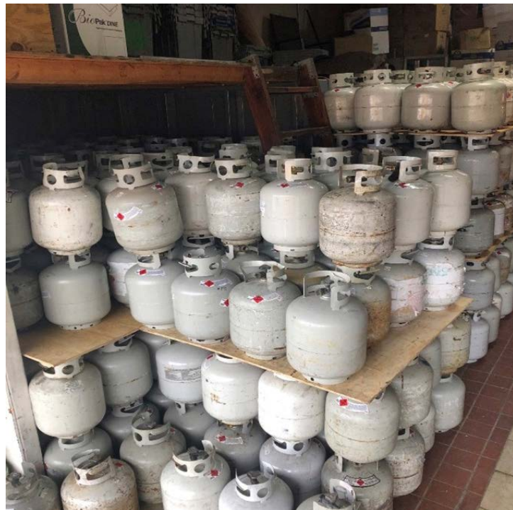
BFP inspectors discovered the unsafe and unlawful storage of more than 900 propane containers at a Brooklyn warehouse in January 2021. Photo credit: Joe Rogers
