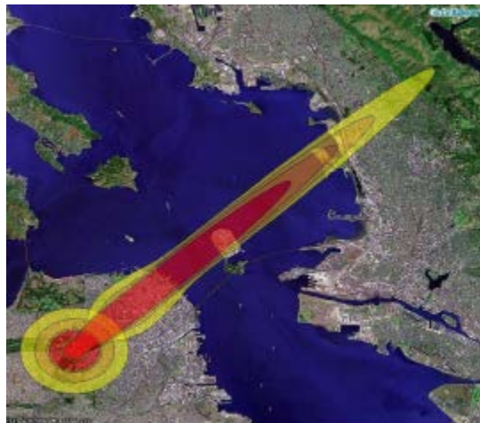
Figure 2. Typical Gaussian “Cigar-Shaped” Plume Model (From Mars, 2007)
