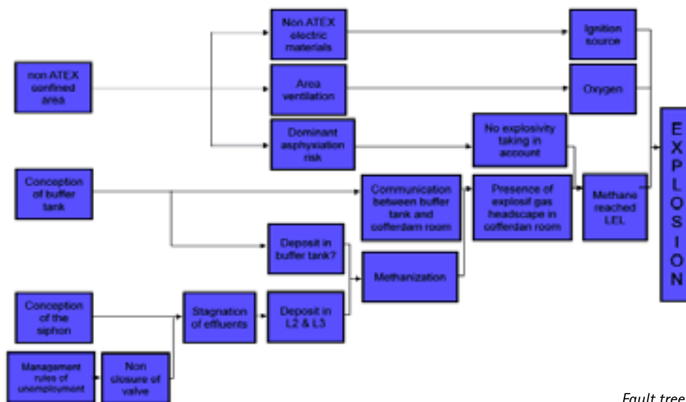
Fault tree of methane explosion
